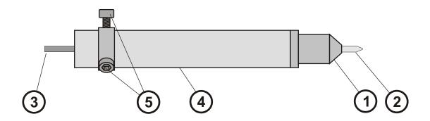
Take the refill holder 4 and release the 3 screws 5. Insert a refill 3 into the holder till the tip 2 exits from the hole 1.
